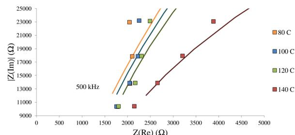
Figure 5: Low frequency Nyquist analysis of phosphoric acid-doped PBI (doping level 2.81) in propiophenone
