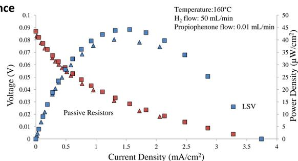
Figure 3: Performance of TRFC1 – comparison of results from passive resistor and linear sweep voltammetry methods
