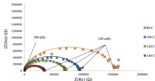
Figure 6: Nyquist analysis of phosphoric acid-doped PBI (doping level 2.81) in propiophenone
