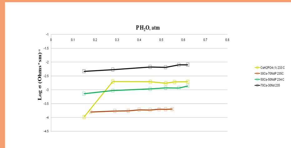
Fig. 3. Conductivity of  $\text{CsH}_2\text{PO}_4$  and mixed composites at temperature approximately 235 C° with different humidity content.
