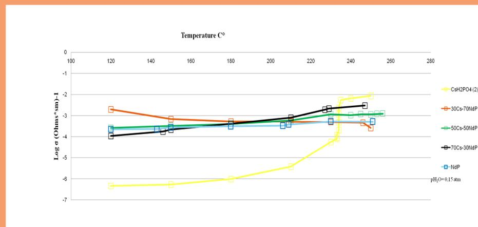
Fig. 2. Conductivity of  $\text{CsH}_2\text{PO}_4$ , mixed composites and  $\text{NdPO}_4 \cdot n\text{H}_2\text{O}$  at different temperatures from 120 C° to 250 C° with constant humidity ( $P_{\text{H}_2\text{O}} = 0,15 \text{ atm.}$ )
