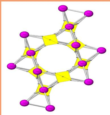
Fig. 1. Structure of  $\text{NdPO}_4$  (rhabdophane structure)
