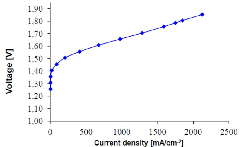
Anode: 1.72mg/cm<sup>2</sup> IrO<sub>2</sub>, Cathode 0.80 g/cm<sup>2</sup> Pt, GDL 0.5mm Ta coated steel felt, Aquivion membrane, 60 µm thick, Temperature 120°C, Pressure 3 bar
