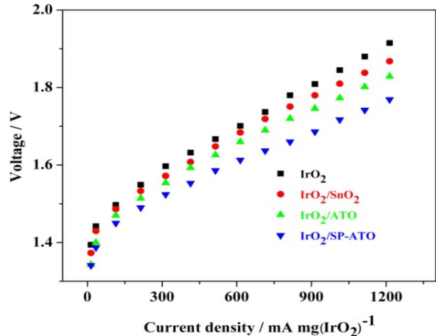
PEM steam electrolysis at 130 °C and atmosphere pressure.
