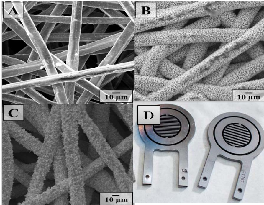
A: Steel felt (uncoated)
