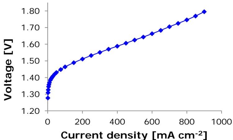
Anode: 0.98 mg/cm<sup>2</sup> IrO<sub>2</sub>, Cathode 0.34 g/cm<sup>2</sup> Pt, GDL 0.5mm Ta coated steel felt, Aquivion membrane, 63µm thick, Temperature 130°C, Atmospheric Pressure
