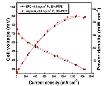
Polarization curves for EPD and Asymtek sprayed MEAs. Pt loading: 0.4 mgcm<sup>-2</sup> with 50% PTFE. Cell temperature 160°C. Gas flow: 0.5 slpm H<sub>2</sub> and 1 slpm air at 0% RH.
