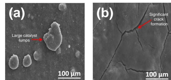
SEM images of (a) Asymtek sprayed GDE (b) EPD GDE. Pt loading 0.4 mgcm<sup>-2</sup> with 50% PTFE. Magnification X1000
