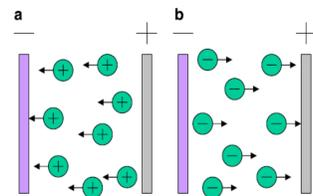
Schematic illustration of electrophoretic deposition process. (a) Cathodic EPD and (b) anodic EPD.
