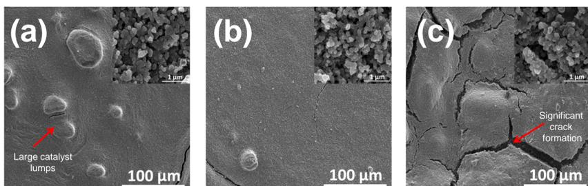
SEM images of (a) hand sprayed GDE (b) Asymtek sprayed GDE (c) EPD GDE. Magnification X1000 and X100 000 (insert).
