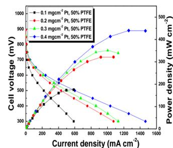
Polarization curves for EPD MEAs. Pt loading: 0.1 - 0.4 mgcm<sup>-2</sup> with 50% PTFE. Cell temperature 160°C. Gas flow: 0.5 slpm H<sub>2</sub> and 1 slpm air at 0% RH.
