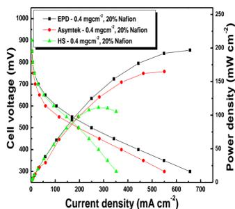
Polarization curves for EPD, hand sprayed (HS) and Asymtek sprayed MEAs. Pt loading 0.4 mgcm<sup>-2</sup> with 20% Nafion. Cell temperature 160°C. Gas flow: 0.5 slpm H<sub>2</sub> and 1 slpm air at 0% RH.
