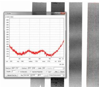
**Figure 4.** Example of the Pt distribution measured across the electrode by X-ray. In this example, the nozzles are moved in the transverse direction during the spraying process in order to average-out the nozzle's individual plume profiles.
