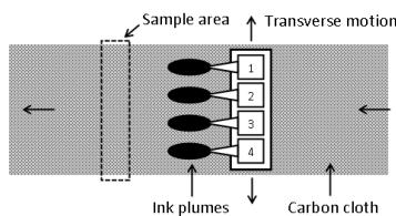
**Figure 2.** Left - A spray coater with four ultrasonic nozzles was used to spray a Pt/C-based catalyst ink onto a 200 cm long, 20 cm wide, rotating carbon cloth belt. The ink consisted of a commercial Pt/C catalyst, dispersed in pure formic acid. Right - Schematic picture of the spraying arrangement.
