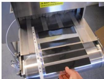
**Figure 1.** Left - The X-ray measurement system from InnospeXion®. Right - Electrode samples at the entrance of the X-ray machine.
