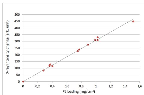
**Figure 5.** A linear relationship between the average Pt loadings and the average grey scale level of the digital X-ray images is demonstrated.
