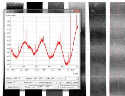
**Figure 3.** Example of the Pt distribution measured across the electrode by X-ray. In this example, the nozzles are fixed in a stationary position during the spraying process.
