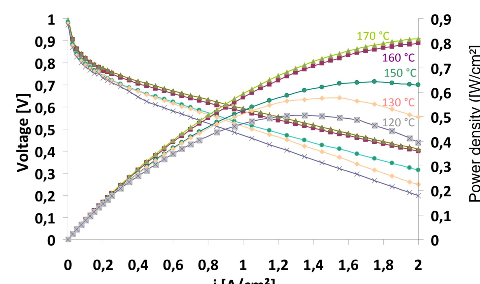
Polarisation curves with cross-linked m-PBI/H<sub>3</sub>PO<sub>4</sub> membrane. Temperature effect with H<sub>2</sub>/O<sub>2</sub>. Baltic Fuel Cell electrodes.
