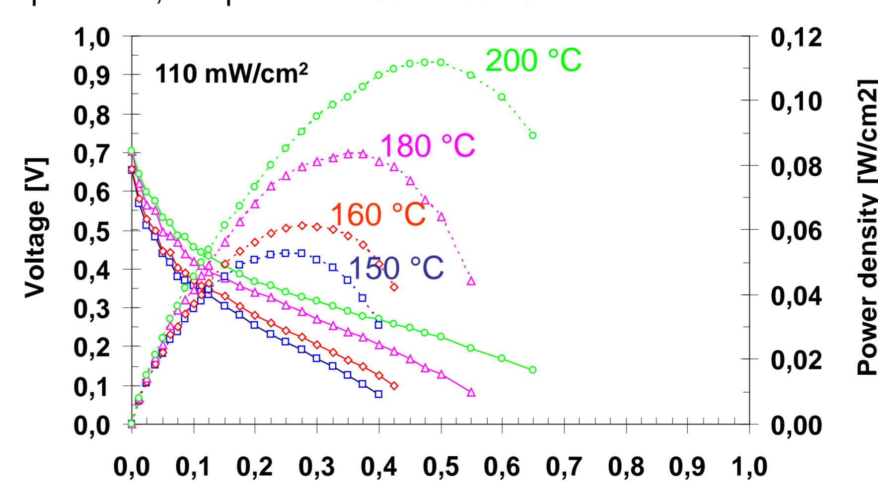
Polarisation curves with cross-linked m-PBI/H<sub>3</sub>PO<sub>4</sub> membrane. Temperature effect with ethanol/water [4.2M] gas mixture/Oxygen. Baltic Fuel Cell electrodes.
