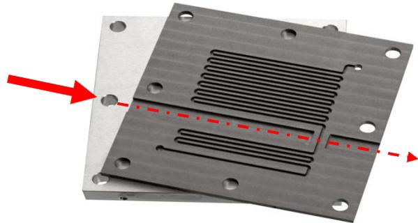
In-plane synchrotron X-ray radiography
