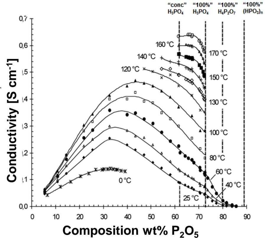
Conductivity as function of composition and temperature
