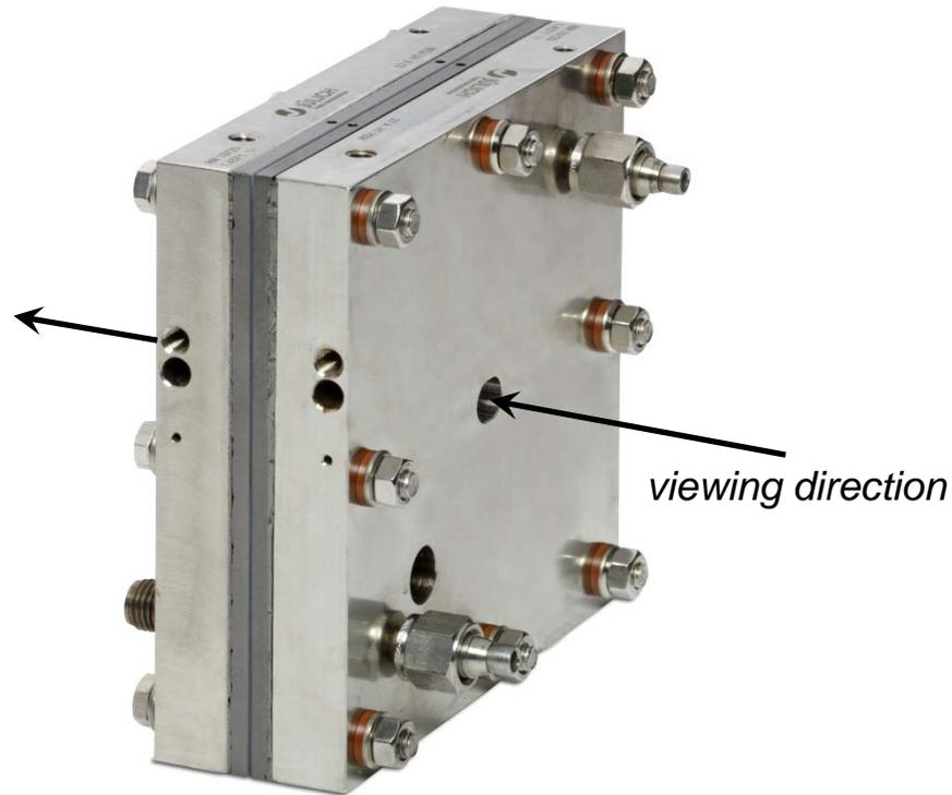
*Assembled measuring cell for through-plane measurements*
