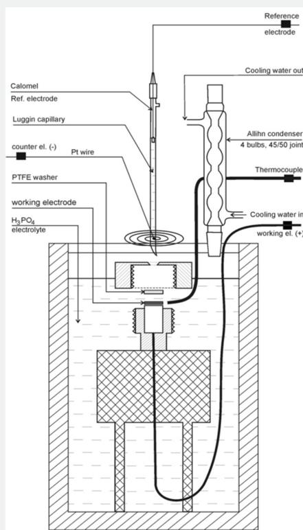
Figure 1. A cell, used to estimate the corrosion resistance of materials<sup>1</sup>.
