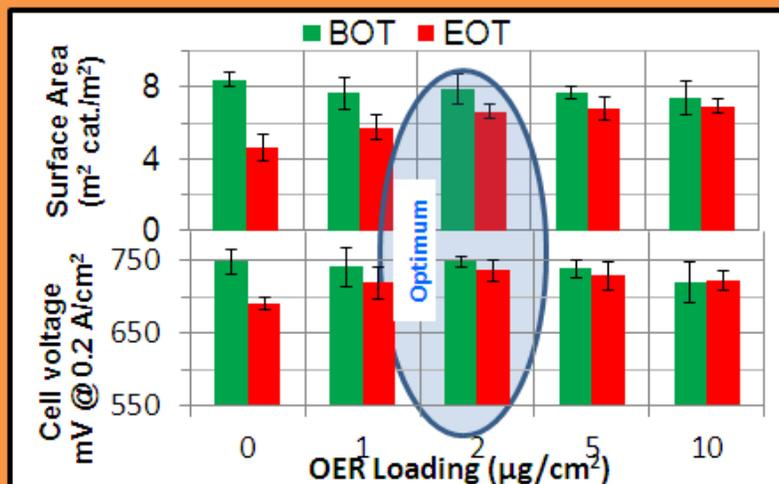
IrRu-modified cathodes have achieved the SU/SD Go/No Go requirement: 5,000 cycles with end voltage < 1.60 V, ECSA loss < 10% with < 0.09 mg/cm<sup>2</sup> PGM
