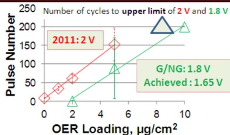
IrRu-modified anodes have achieved the cell reversal Go/No Go requirement: 200 cycles with end voltage < 1.80 V, with < 0.045 mg/cm<sup>2</sup> PGM
