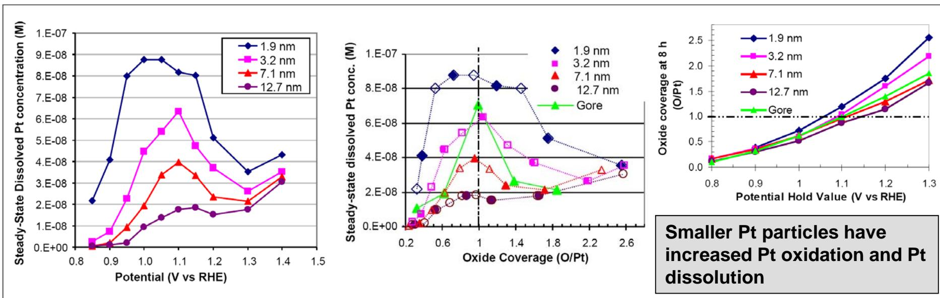
**Smaller Pt particles have increased Pt oxidation and Pt dissolution**
