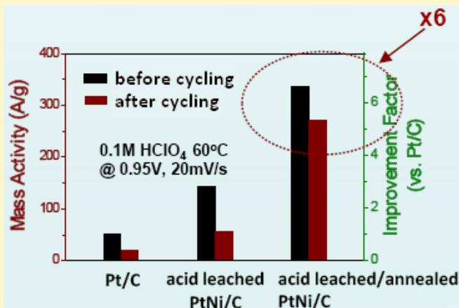
**Performance:** Nanosegregated PtNi/C catalysts have ORR mass activity 6X that of Pt/C in RDE testing.
