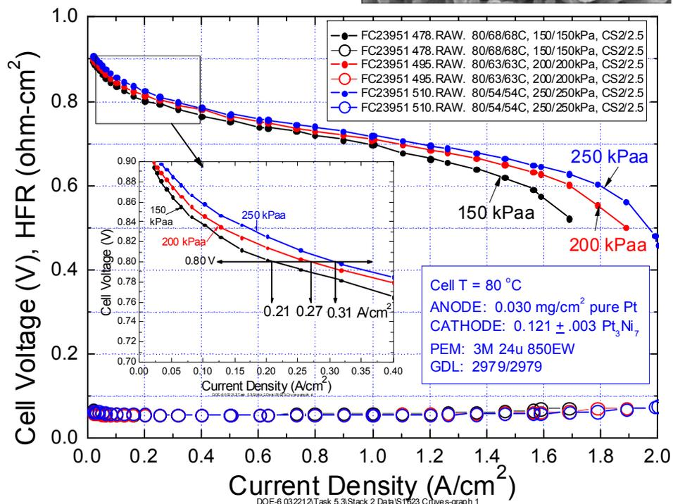
**New 3M project will improve MEA components and optimize component integration to simultaneously achieve catalyst, membrane, and MEA targets**
