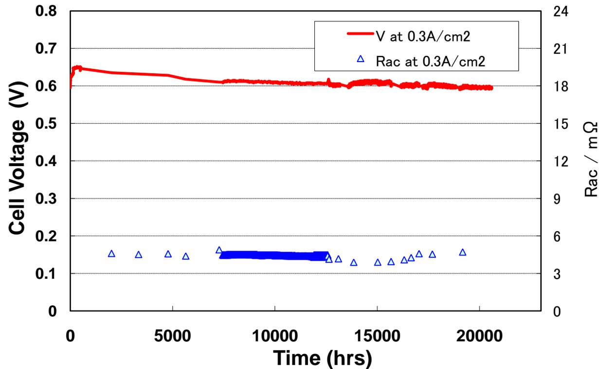
25 cm<sup>2</sup> cell, 150 °C, H<sub>2</sub>/air, operated at 0.3A/cm<sup>2</sup>
