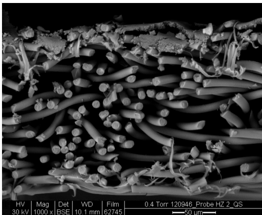
GDS Development - SEM, cross section, MPL on upper side (FILK, M. Langer)
