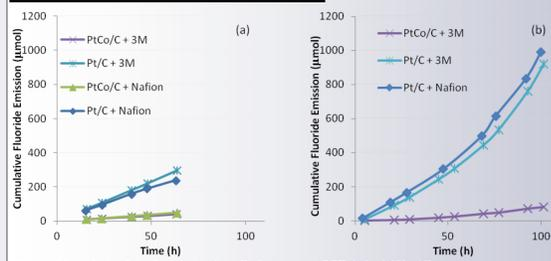
Figure 4 Cumulative fluoride emission for cells that were (a) PET & (b) OCV AST
