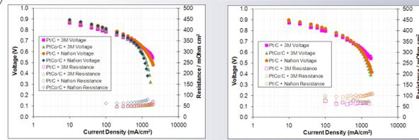
Figure 2. Performance at 80 °C/100% RH at BOL before PET. Figure 3. Performance at 80 °C/100% RH at BOL before OCV AST.
