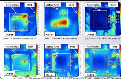
Figure 6. IR images of tested MEAs. Temperature increases are noted with approximate temperatures based on the emissivity of carbon.
