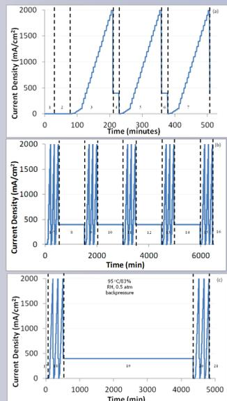
Figure 1. (a) Current density vs time for ~24 h of testing; (b) Current density vs time for the performance portion of testing; (c) Current density vs time for the stability portion of testing. The cell is shutdown between the performance and stability portions of testing. Numbers refer to Table 1.
