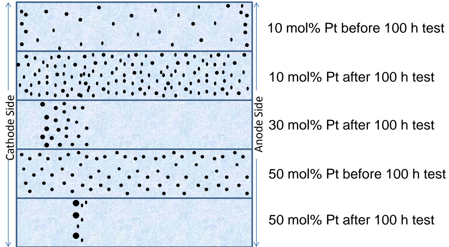
❖ After testing, 10 mol% Pt had smallest particle distance and size, and the greatest overall Pt coverage
