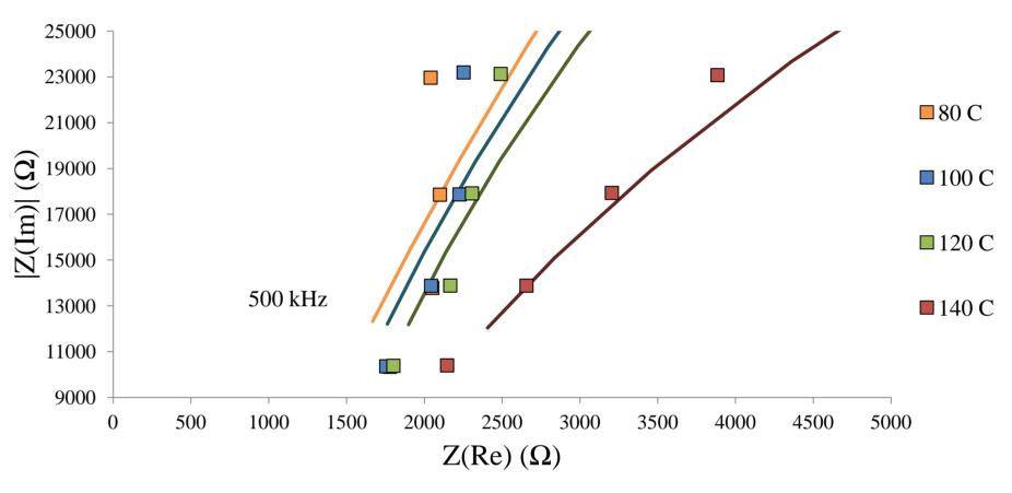
Figure 5: Low frequency Nyquist analysis of phosphoric acid-doped PBI (doping level 2.81) in propiophenone
