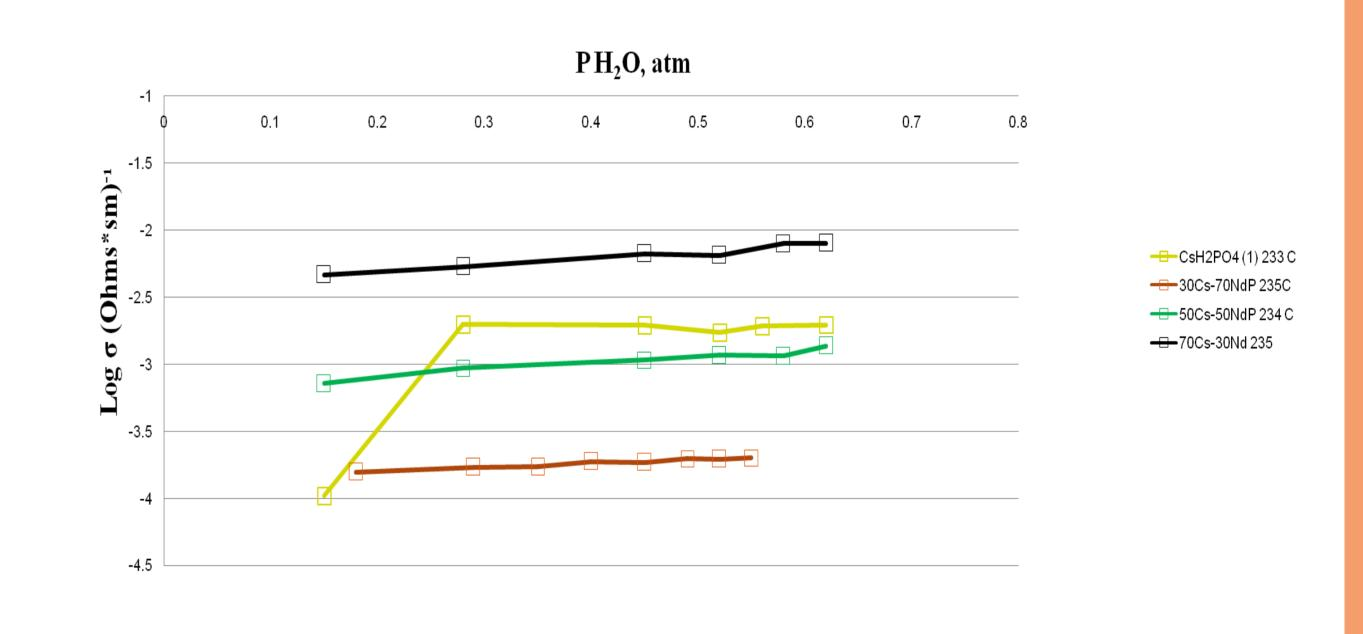
**Fig. 3**. Conductivity of  $CsH_2PO_4$  and mixed composites at temperature approximately 235 C° with different humidity content.
