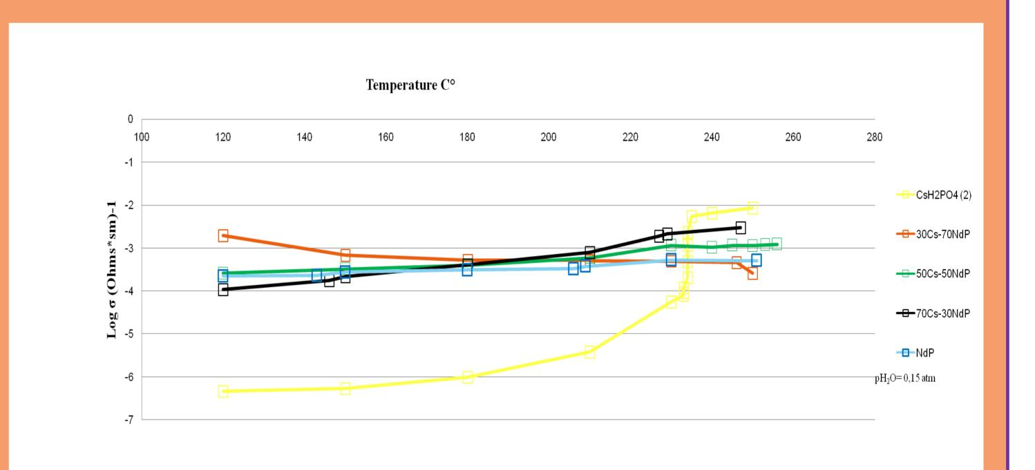
**Fig. 2.** Conductivity of  $CsH_2PO_4$ , mixed composites and  $NdPO_4 \cdot nH_2O$  at different temperatures from 120 C° to 250 C° with constant humidity  $(P_{H2O}=0,15 \text{ atm.})$
