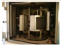
PVD (Physical Vapor Deposition) is a well-known technology in other sectors such as microelectronics that could be applied to concentrate the catalyst layer closer to the membrane and reduce the Pt specific load.
