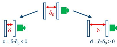
2. Constant displacement  $\rightarrow$  Contact pressure (P<sub>c</sub>) as measured variable
