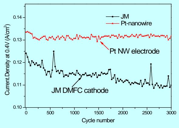
75 °C, 3000 loading cycles: 0.2–0.7V, 50 mV s<sup>-1</sup>, Anode: 1.0 mL min<sup>-1</sup> 1N CH<sub>3</sub>OH; Cathode: 100 sccm air
