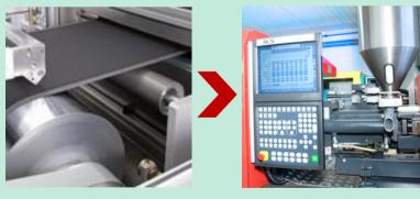
Electrode manufacturing Lamination & gasket Capacity: 20.000 sqm/yr using injection molding
