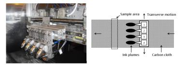
**Figure 2**. *Left* - A spray coater with four ultrasonic nozzles was used to spray a Pt/C-based catalyst ink onto a 200 cm long, 20 cm wide, rotating carbon cloth belt. The ink consisted of a commercial Pt/C catalyst, dispersed in pure formic acid.
