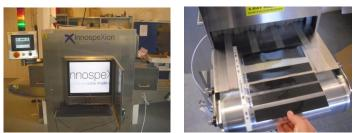
**Figure.1**. *Left* - The X-ray measurement system from InnospeXion<sup>®</sup>. *Right* - Electrode samples at the entrance of the X-ray machine.
