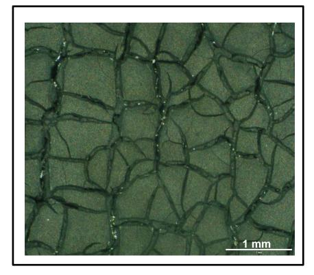
*Microscope image of a gas diffusion electrode after the drying step over night.*
