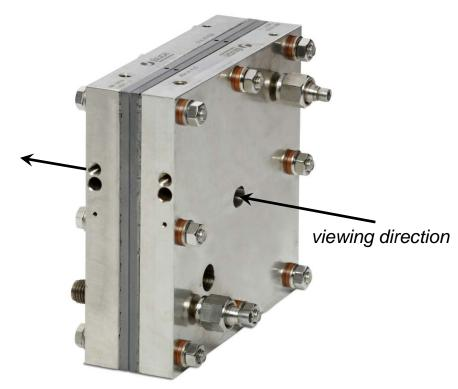
Assembled measuring cell for through-plane measurements
