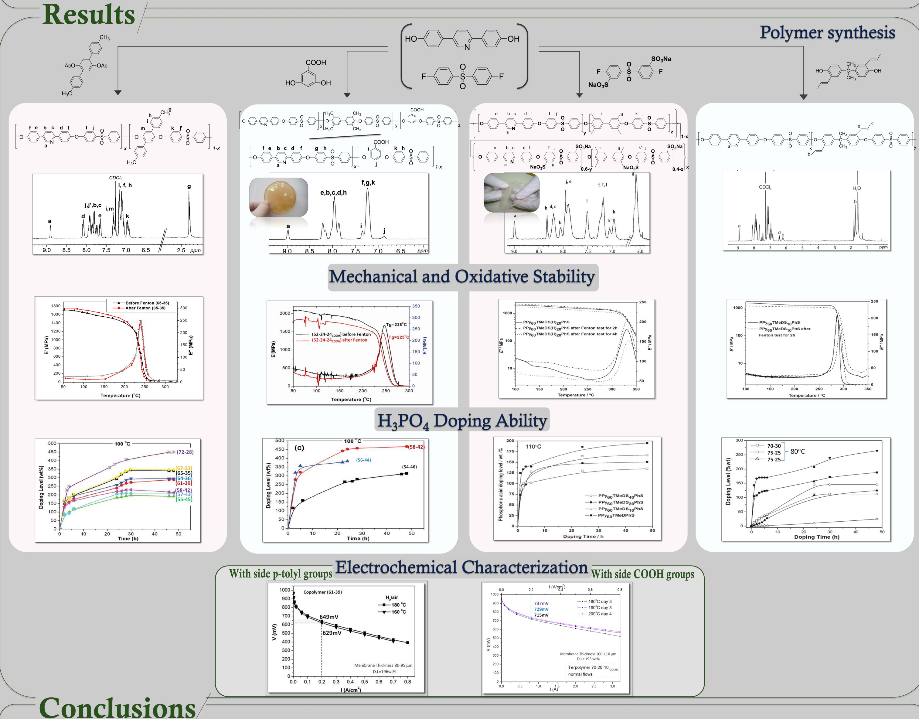
Copolymers bearing main chain pyridine units and p-tolyl, carboxyl, sulfonic units and double bonds as side groups were synthesized with high molecular weight, excellent mechanical and thermal properties, increased  $H_3PO_4$  acid uptake.
