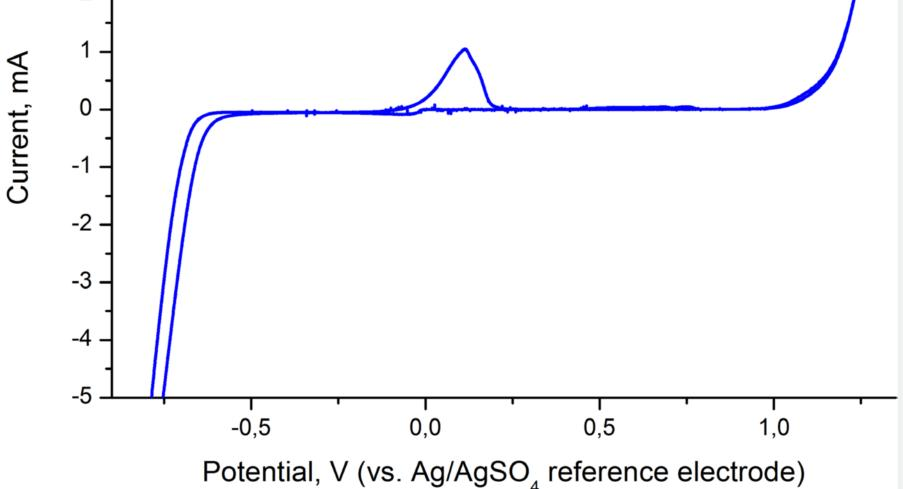
Figure 2. The voltammetric curve obtained on Pt.
