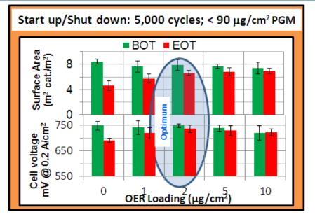
IrRu-modified cathodes have achieved the SU/SD Go/No Go requirement: 5,000 cycles with end voltage < 1.60 V, ECSA loss <10% with < 0.09 mg/cm<sup>2</sup> PGM Cell Reversal: 200 x 0.2 A/cm<sup>2</sup> w/ 45 μg/cm<sup>2</sup> PGM
