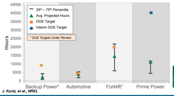
PEM & SOFC data from lab tested, full active area short stacks and systems with full stacks. Data generated from constant load, transient load, and accelerated testing.
