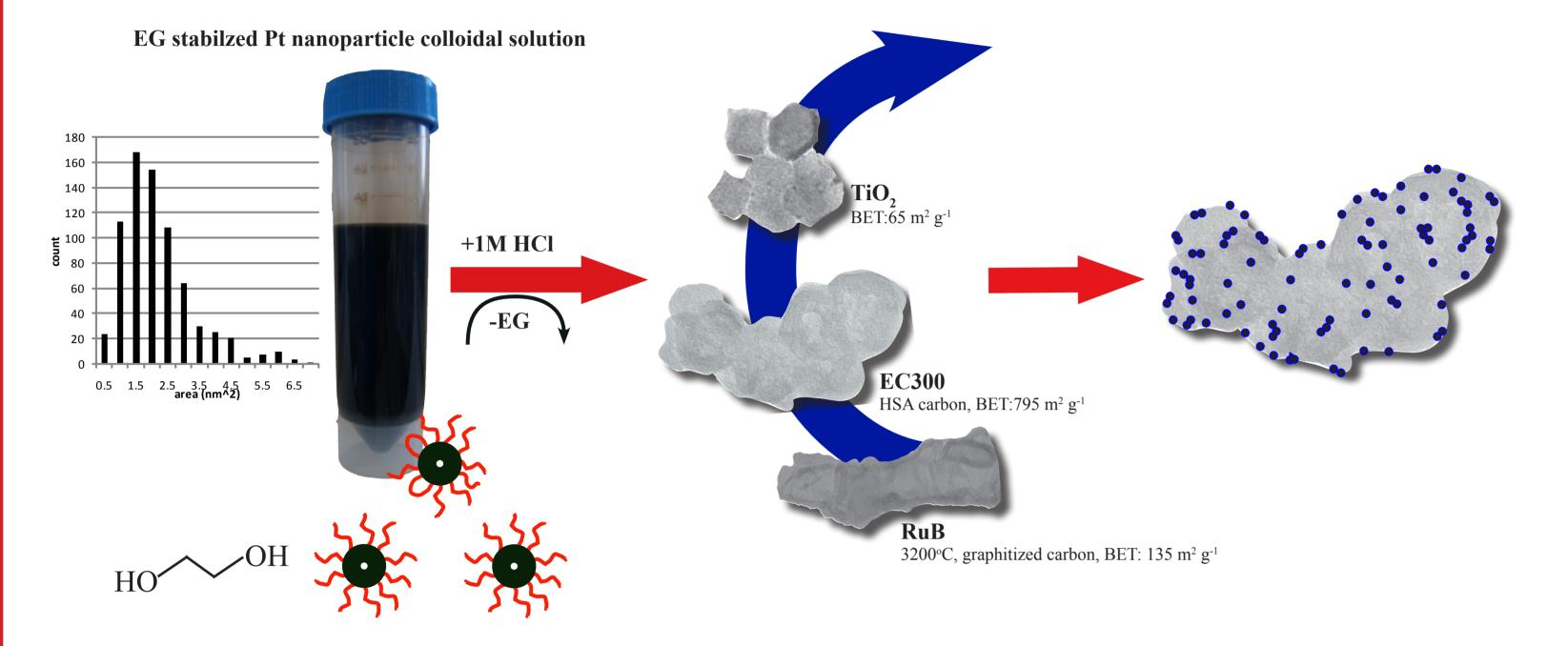
The ethylene glycol (EG) method allows us to produce small metal particles with a narrow size distribution. It is a very powerful method to produce catalysts, because it enables us a controlled synthesis of catalysts where individual parameters such as particle size, support material and Pt loading can be tuned without changing other parameters.
