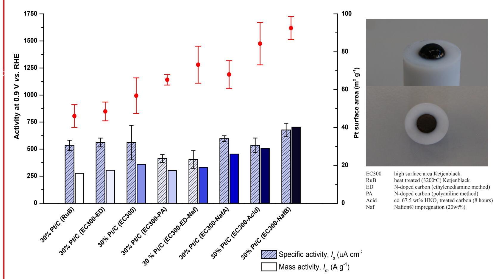
Comparison of specific  $(I_s)$  and mass  $(I_m)$  activities of model catalysts for ORR in 0.1 M HClO<sub>4</sub>, determined at 0.9 V vs. RHE
