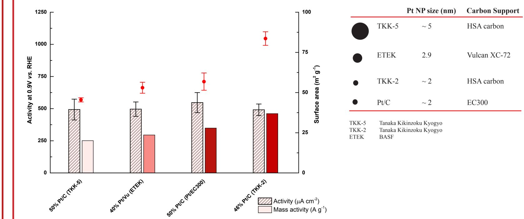
Comparison of specific  $(I_s)$  and mass  $(I_m)$  activities of commercial and model catalysts for ORR in 0.1 M HClO<sub>4</sub>, determined at 0.9 V vs. RHE
