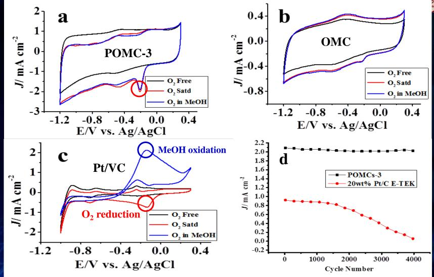
CVs for POMC-3 (a), undoped OMC (b), and commercial Pt (20 wt%)/VC catalysts (c) at different conditions. ORR peak max currents for POMC-3 and commercial 20 wt% Pt/VC catalysts during the repeated potential cycling (d).
