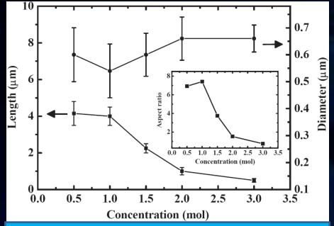
Effects of HCl concentration on length and diameter of SBA-15 particles. Inset represents the aspect ratios of the SBA-15 particles as a function of HCl concentration.
