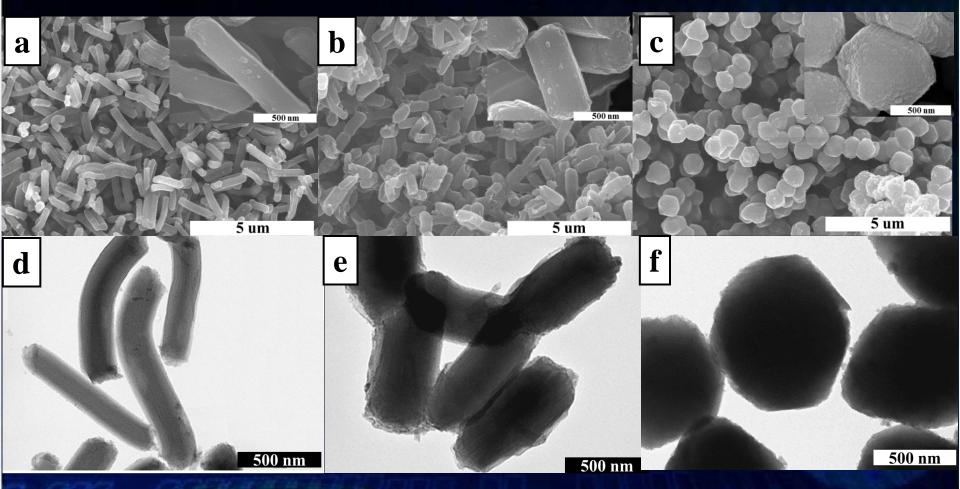
FE-SEM and TEM images of POMCs with different sizes: (a, d) POMC-1, (b, e) POMC-2 and (c, f) POMC-3. (length of 1.5, 1.0, and 0.7  $\mu$ m and thickness of 0.2, 0.4, and 0.8  $\mu$ m, respectively) Carisma 2012 – 3rd Carisma International Conference 🔣
